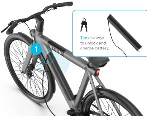
**Tip:** Use keys to unlock and charge battery.
